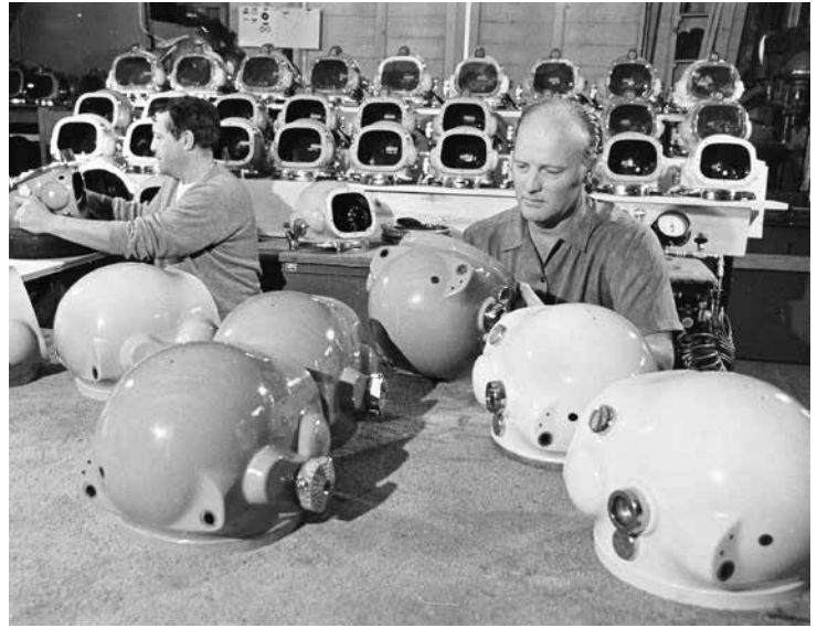
Cal Dive's Secret Weapon: Developed by founder Bob Ratcliffe, the Rat Hat system was uniquely able to keep a diver warm under arctic conditions, keep him secure surface diving to helium depths and flexible enough for lock-out bell diving. Such safety-oriented equipment gave Cal Dive a leg up on attracting top divers and a real advantage in accomplishing difficult tasks. Rat Hats were not for sale. Kirby-Morgan headgear is now the gold standard. Oceaneering still features the Rat Hat emblem.
